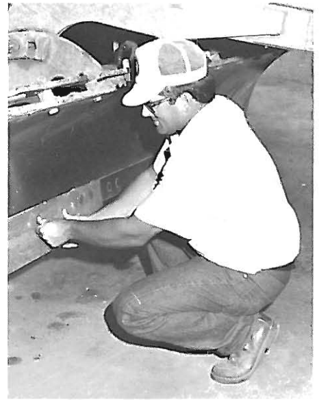
Freddie Fight, an 11 veteran of the Department, changes blades on a motor grader.
